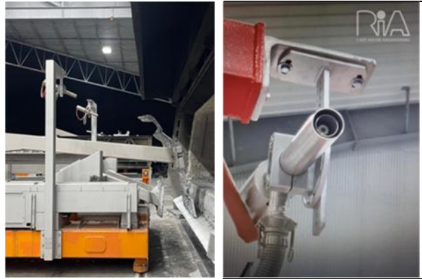
Figure 4. Air-Cooled smart camera technology for high temperature applications, onboard a rail-mounted skimming machine.
