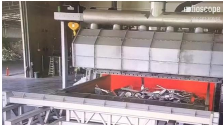
Figure 2. On-board camera monitoring the furnace charging cycle, relaying the footage to operators who can be situated in the safety of the operator pit.
