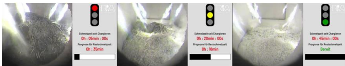
Figure 1. Screenshots of AI system smart cameras relaying real time information of melt progress to the cast house.
